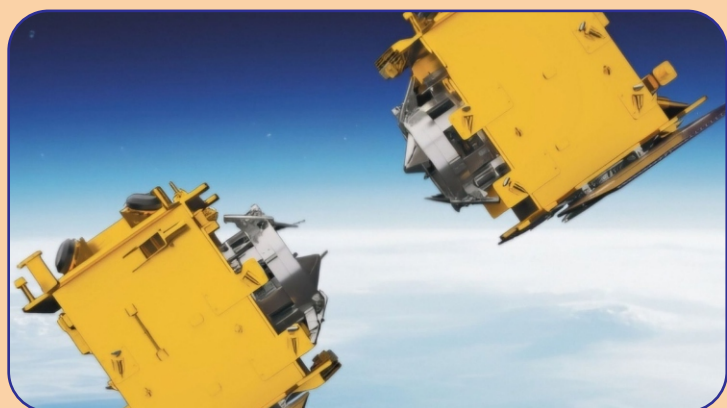
Illustration of the two SpaDex Satellites just before and after docking. Image credit – Indian Space Research Organization (ISRO).
